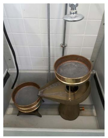
Figure 14. Fenwick can, in use to extract cyst nematodes from wet soil.
