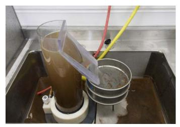
Figure 15. Wye washer, an elutiator for extraction of cyst nematodes from wet soil.
